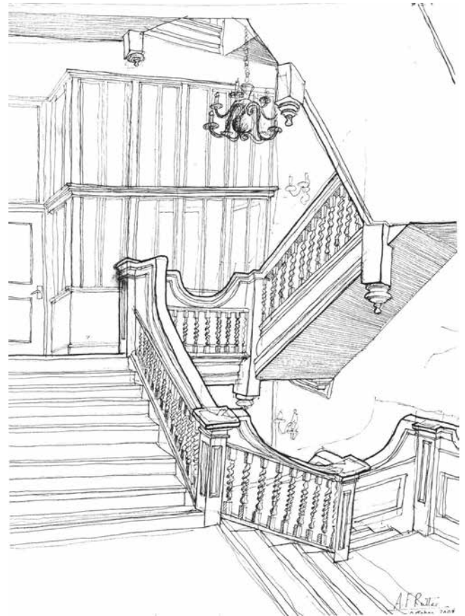
Original main staircase of No. 9, Parchment Street, showing the continuation up into the attic and the new firescreen with 'Pyran' glass..
