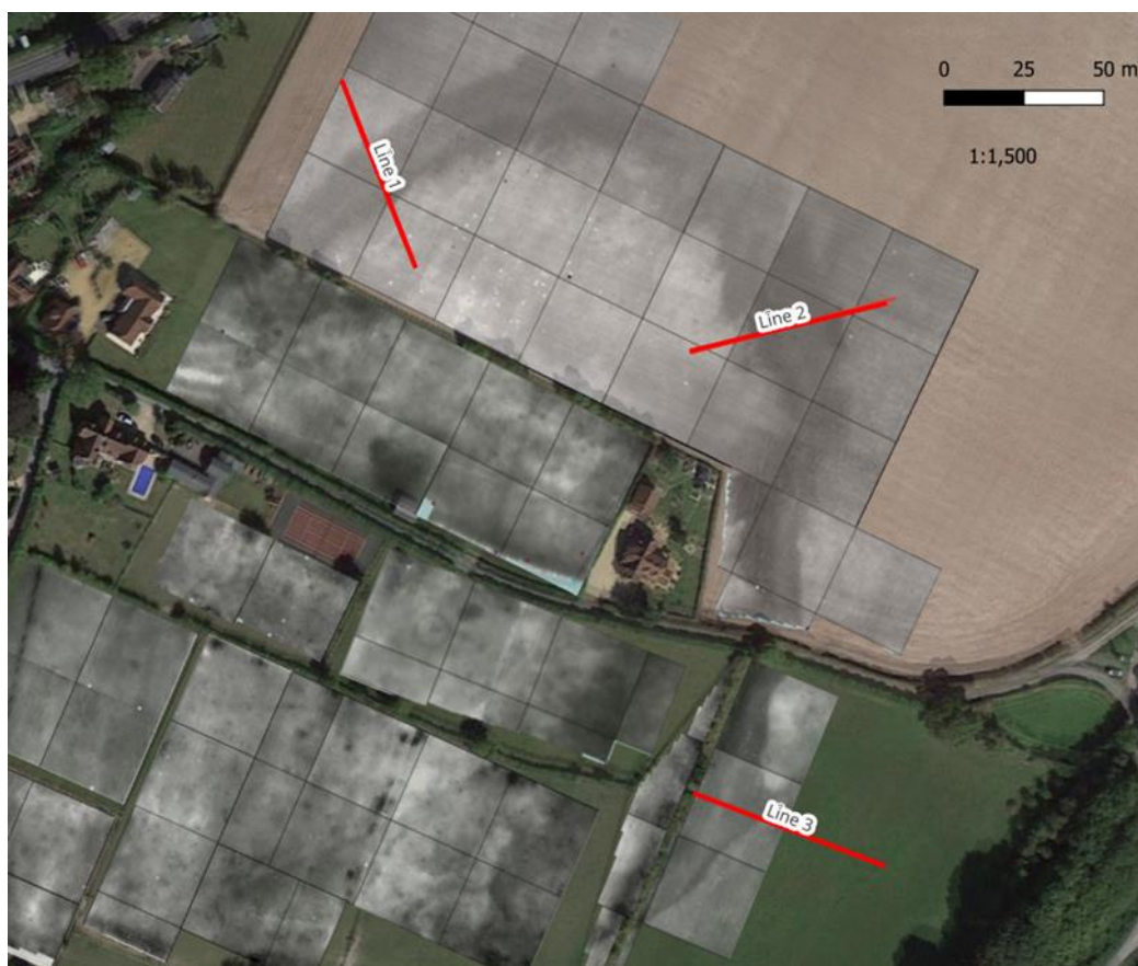
Fig 14 Stocks Lane: Electrical Resistivity Tomography survey lines and resistivity results superimposed over Google imaging
